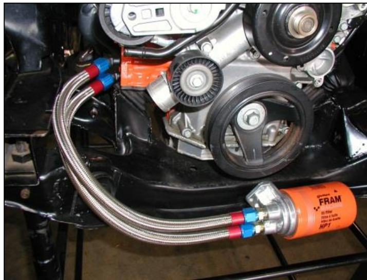
Remote filter mounted for illustration purposes only. Mount your filter to suit your application.
